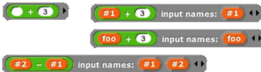
The names **#1**, **#2**, etc. are provided by default, but you can change a name by clicking on its orange oval in the **input names** list. Be careful not to *drag* the oval when clicking; that's how you use the input inside the ring. The names of the input variables are called the *formal parameters* of the encapsulated procedure.
